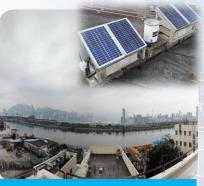
Rain Gauge for Slope Monitoring
