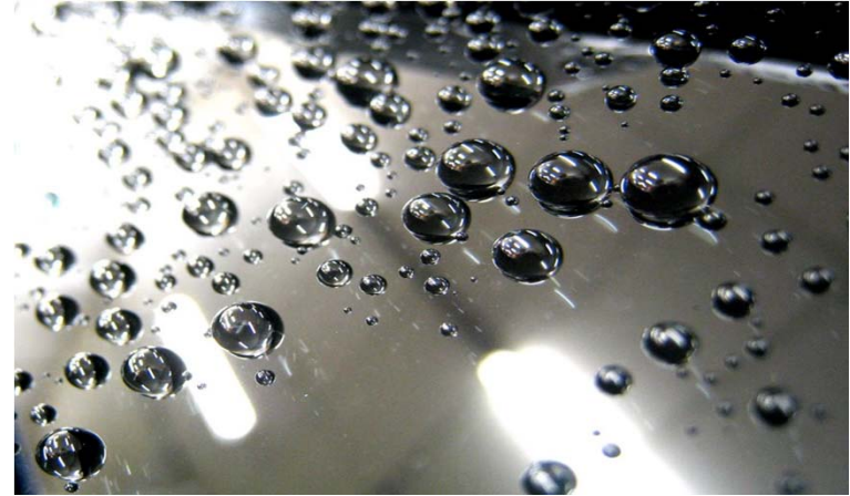
Super-hydrophobic self-cleaning glass
